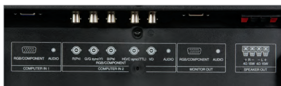
Analog computer and video inputs accessible from the bottom of the display.
